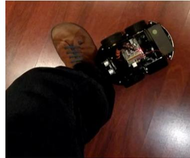
Figure 4 - The Robot4All Car stops when it detects an obstacle
